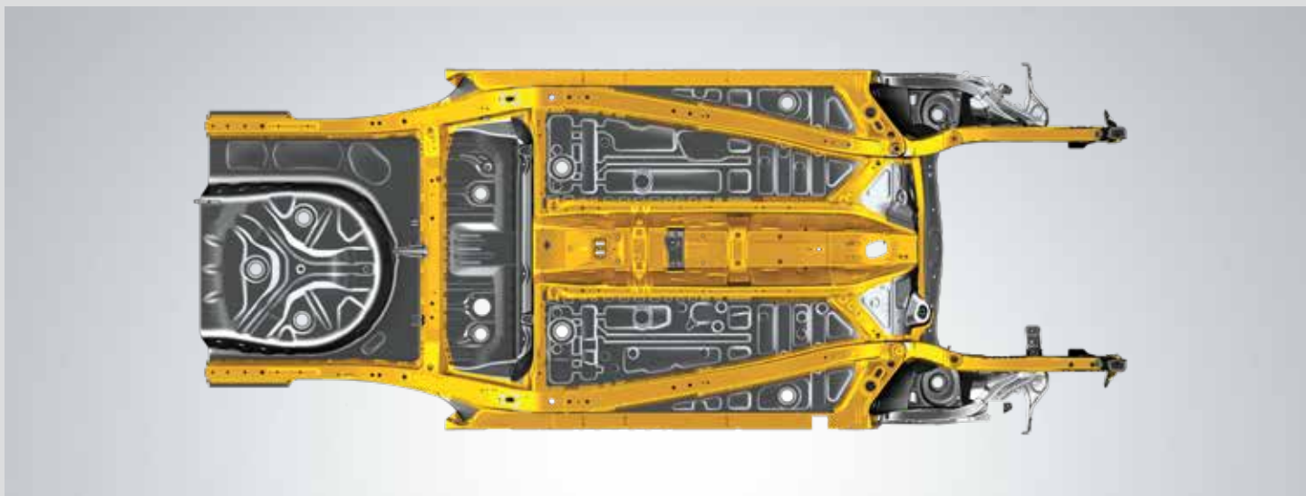
Suzuki HEARTECT Platform Absorbs collision impact, enhances safety
